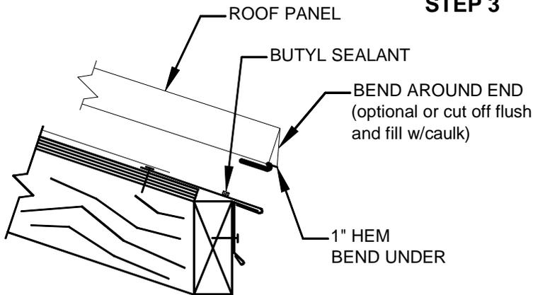
6. Mark 1" in pan of panel and cut beside each rib with a tin snips.
