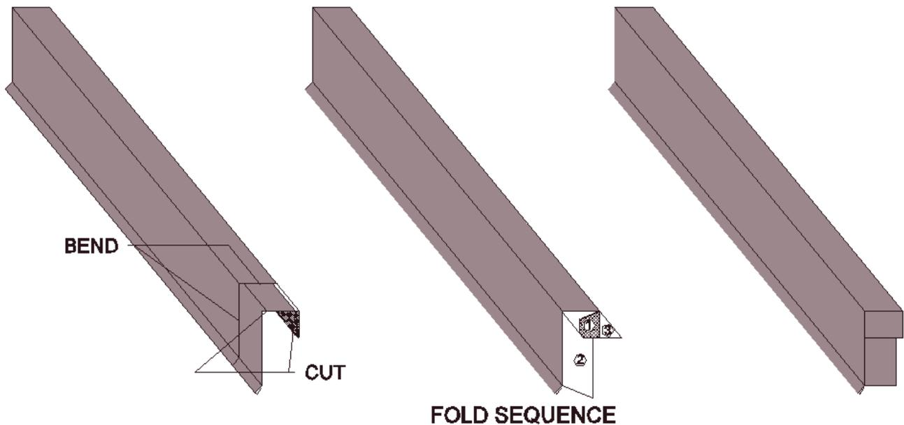
**After snapping the gable flash over the cleat, pull the gable flash over the eave end fascia by 2" to 3" to finish fold. See diagram for cuts and bending locations. Always fold the sides in first and fold the top flap down last so water will run off and NOT run in.**
