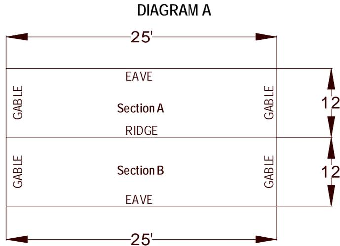
The length from the eave to the ridge is 12'. The length of the ridge is 25'; therefore, the number of panels to complete one side of the house is  $25' \div 1.33'(16'') = 19$  pcs. Your materials list should look like Sample B.
