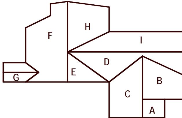
B. Sketch a diagram of each roof section. Show all measurements (see example below.) **It is important to measure the exact center of the ridge to the eave edge.** Do not allow anything for overhang.
